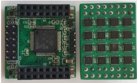
Figure 3 The complete module with 16 IMU sensors
