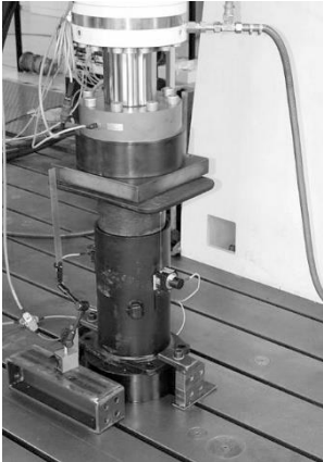
Fig. 1. Railway buffer during measurements in the ERCT dynamic test lab
