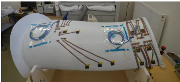
Fig. 4. Right air inlet with installed sensors.
