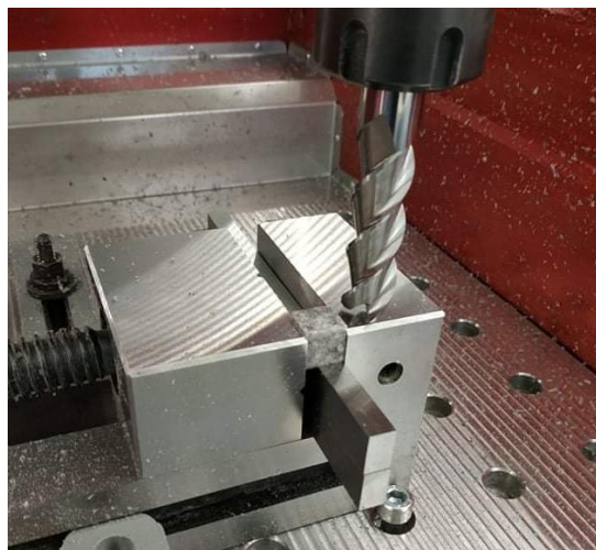
Fig. 1. Machining a foam specimen
