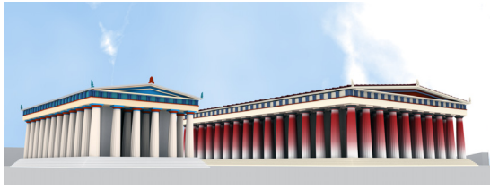
(b) A peripteral and a dipteral temple generated with the same grammar
